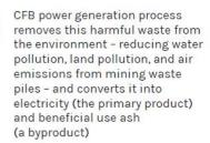
CFB fuel mix neutralizes sulfur dioxide (SO<sub>2</sub>) with limestone and creates a calcium-rich, basic (high-PH) ash, most of which is currently returned to mining waste piles to reclaim land, facilitating revegetation
